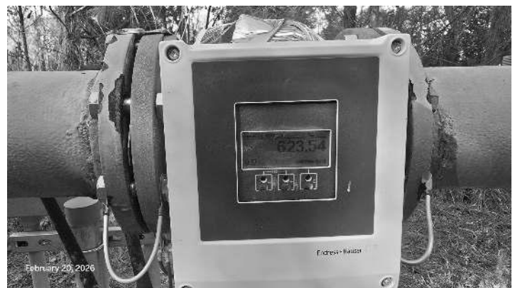
Field Photograph of flow meter reading 23.4 gons per minute
